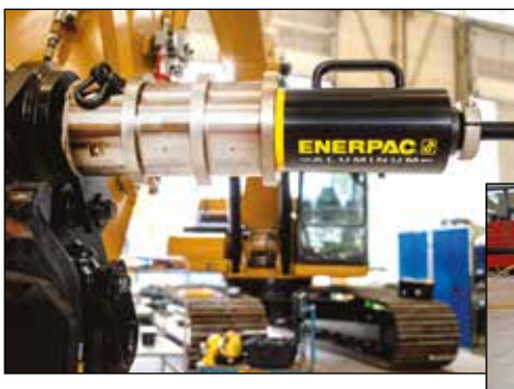
◀ Excavator maintenance using the PPH40 powered by a SC-Series Cordless Pump.
