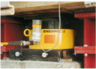
High Tonnage Cylinders Capacity: 50 - 1000 ton
